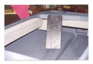
The entire floatation system of the boat has been redesigned with rail mounted, foam filled ABS Floatation Tanks. There is an ABS piece designed to fit the stern to encapsulate the urethane floatation foam along with the poured foam in the bow. This gives us even more floatation than is required and provides you with an added margin of safety should it ever be needed. During assembly, you may also add/have added an optional S/S tow/anchor eye.
